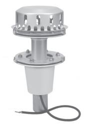
Heated roof drains can be connected in individual switching or parallel connection. The automatic central control takes place via an outdoor thermostat (for large plants hygrostats are additionally used) and two-point controllers. The necessary components are customary, e. g. from the area of the heating control system. Heatable roof drains may not be cut to length or changed on site.
